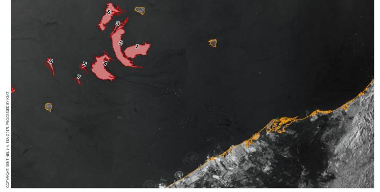
An oil slick is detected in the satellite image and our expert analysts prepare a comprehensive report including information about the spill; time, exact position, extent, confidence level and possible source that is delivered to the end user in NRT.
